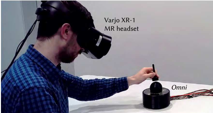
FIGURE 6.9: We combine Omni with a video see-through MR device (Varjo XR-1) to showcase the applications.
