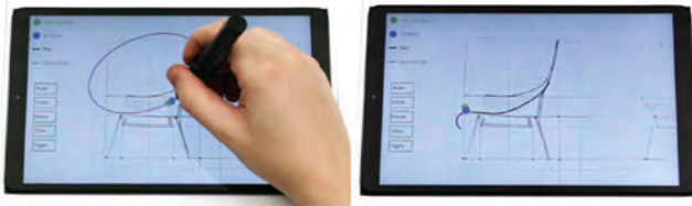
FIGURE 8.11: Virtual tools can be used to dynamically construct a reference path combining haptic and visual feedback. Here a simple drawing application combines freeform sketching with different virtual rules and guides that can be felt by the user.
