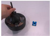
Omni [Langerak2020a] (above) is an haptic device. A symmetric electromagnet is used in combination with a dipole magnet model and a simple control law to deliver dynamically adjustable forces onto a hand-held tool. The tool only requires an embedded permanent magnet and thus can be entirely untethered. Here the haptic feedback is elicited on the tool, while the user interacts with the tool. Omni showed that **physical joint interfaces provide more intuitive and accurate user inputs.**
